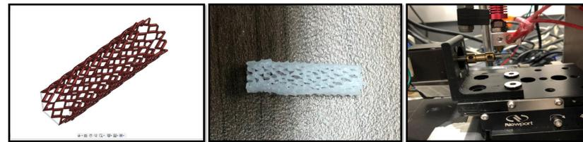
Figure 3: Left: PCL Flow Diverting Stent CAD Design. Middle: PCL 12mm FDS Right: Electromelt PCL Printer with Micromotion platform
